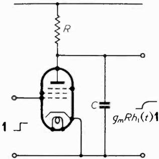
Fig. 1. Simple resistance-coupled stage.
