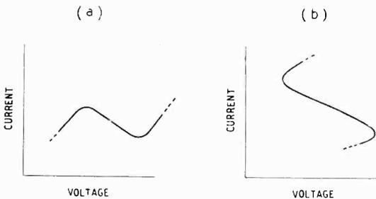
Fig. 1. Negative-resistance characteristic due to voltage control (a) and current control (b).
