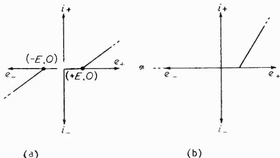
Fig. 4. Symmetrical modified characteristic of a positive resistor (a), unilateral modified characteristic (b).
