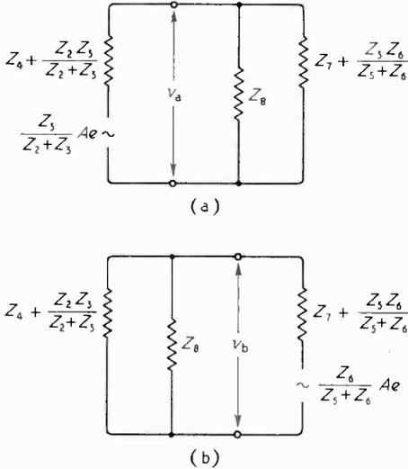
Fig. 3. Reduction of circuit of Fig. 2 by the super-position theorem.
