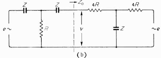
The reason for the above form is that the determinant of the network is also most neatly expressed when multiplied by  $(4R + Z)$ . Hence the numerator of the partial response is given by the right-hand side of Equ. (4) and the other partial response is found in a similar manner.
