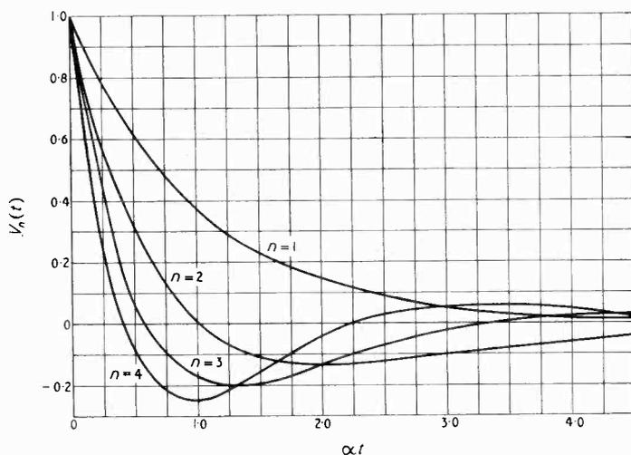
an amplifier with  $n$  identical tuned circuit stages to an input of their natural frequency, modulated by a unit step, is also given by equation (4), where  $\alpha = 1/2RC = \omega_0/2Q$ . The response can therefore be rapidly determined by means of the tables or charts.
