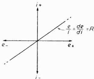
Fig. 3. Characteristic of ideal positive resistor.
