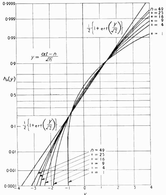
Fig. 3. Response to a unit step of a resistance-coupled  $n$ -stage amplifier.
