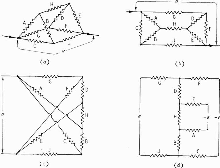
Fig. 7. Variant of "cube of one-ohm wires" (a); squashed flat (b); re-arranged (c) and brought to its final form with independent generators (d).
