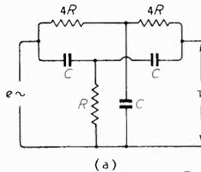
Fig. 5. Parallel-T RC network (a) and its equivalent circuit (b).
