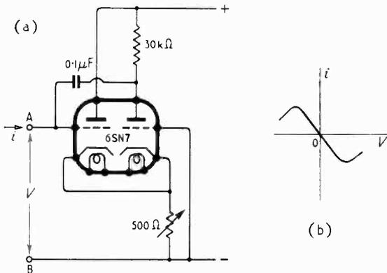
Fig. 6. (a) Cathode-coupled negative-resistance circuit and (b) static  $i/V$  characteristic at input terminals A and B.
