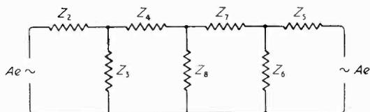
Fig. 2. Equivalent circuit of Fig. 1.
