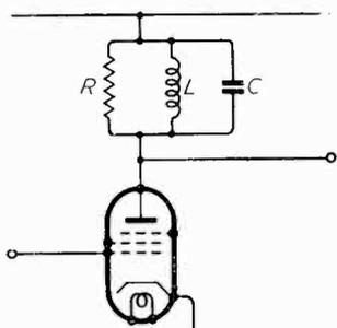
Fig. 4 (above). Single tuned-circuit coupling.
