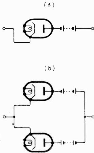
Fig. 6. Illustrating the use of diodes to obtain the characteristic of Fig. 4.
