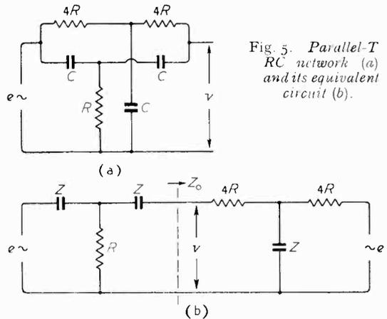
Fig. 5. Parallel-T RC network (a) and its equivalent circuit (b).
