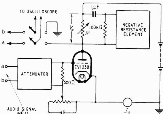
Fig. 7. Diagram of measuring equipment.
