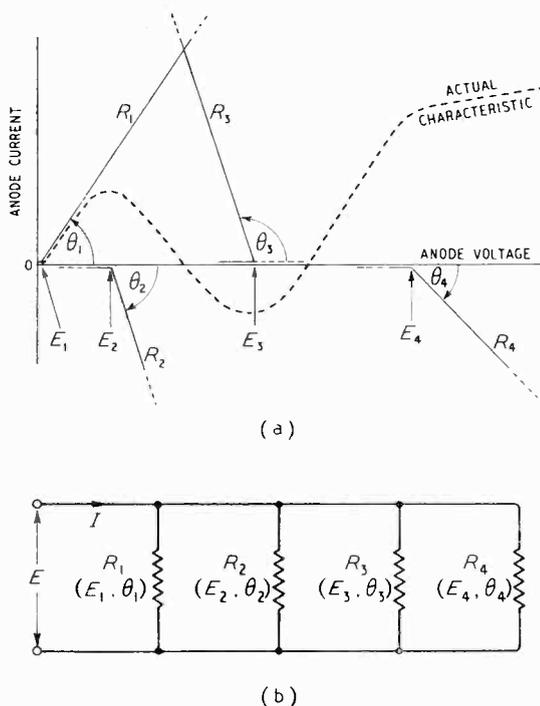
Fig. 5. First-order synthesis of negative-resistance characteristic (a), and equivalent circuit (b). Where  $|\theta| > \pi/2$  [cf.  $R_3$ ] it must be regarded as the resultant of two or more parallel components for each of which  $|\theta| < \pi/2$ ; this case should be avoided by taking the turn in two steps.
