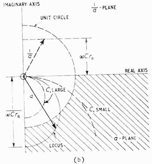
Fig. 5. (a) and (b) show respectively the vector loci of  $1/a$  and  $a$ , for  $R_L$  varying and an assumed shunt capacitance  $C$ , (stage gain is proportional to  $a$ ). The shaded region in (b) shows the area in which gains greater than  $\mu$  occur.
