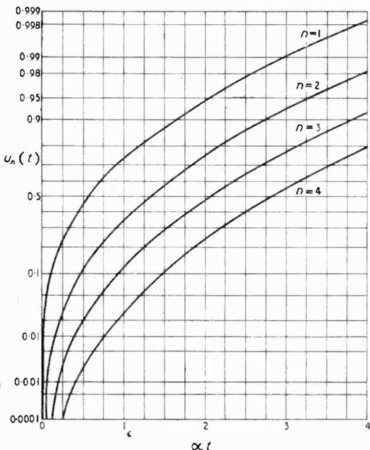
Fig. 8. Response to a unit step of a critically-damped inductance-compensated  $n$ -stage amplifier.
