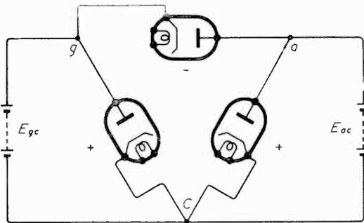
Fig. 8. Diode equivalent circuit of a triode valve. The hypothetical "negative" diode assumes such an impedance value that the required operating condition (usually zero current) obtains in the grid-cathode circuit.
