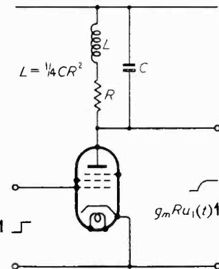
Fig. 7. Critically-damped inductance-compensated stage.
