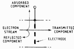
Fig. 7. The components of electron current in a valve are shown.
