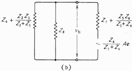
Fig. 3. Reduction of circuit of Fig. 2 by the super-position theorem.
