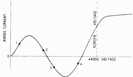
Fig. 2. Characteristic of a screen-grid valve at constant control-grid voltage.
