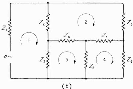
Fig. 1. Parallel-connected T networks (a) and their meshes (b).
