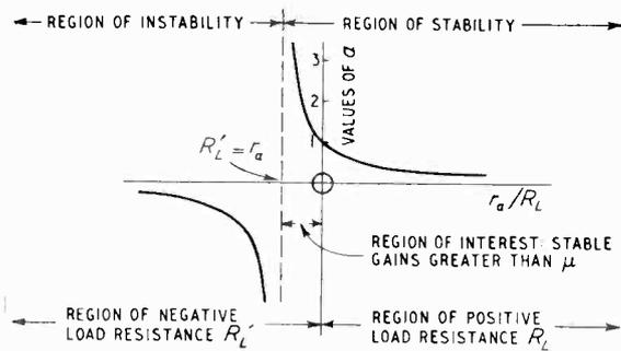
Fig. 2. Relation of normalized amplification  $a$  to  $r_a/R_L$ .
