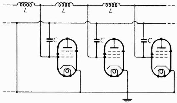
Fig. 9. Filter-coupled amplifier.
