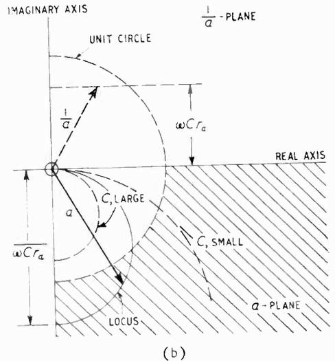
Fig. 5. (a) and (b) show respectively the vector loci of  $1/a$  and  $a$ , for  $R_L$  varying and an assumed shunt capacitance  $C$ , (stage gain is proportional to  $a$ ). The shaded region in (b) shows the area in which gains greater than  $\mu$  occur.
