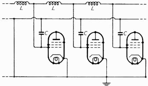
Fig. 9. Filter-coupled amplifier.
