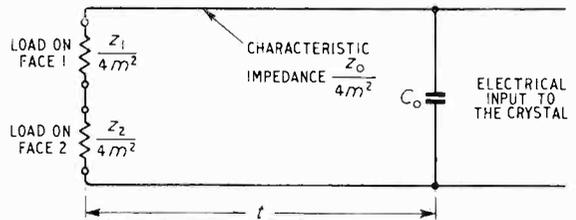
Fig. 2. Equivalent transmission-line circuit for the crystal near resonance.
