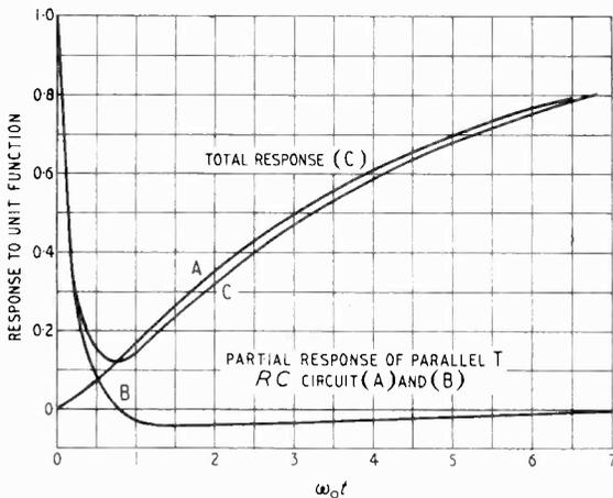
Fig. 6. Partial and total responses of the network of Fig. 5 to a unit step.
