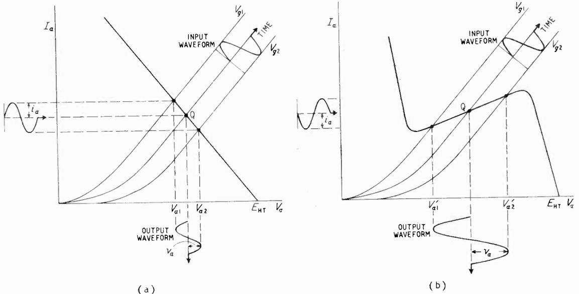
Fig. 1. Load-line diagrams (a) with positive- and (b) with negative-resistance loads. The anode currents are in opposite phase.
