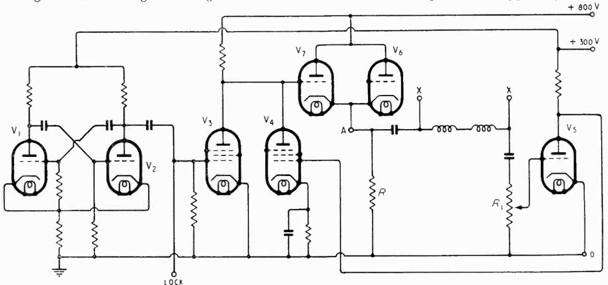
Fig. 4. Elaborate switch circuit including a feedback circuit with which the coil resistance can be cancelled.
