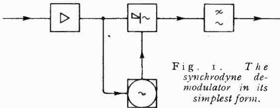
Fig. 1. The synchronous demodulator in its simplest form.
