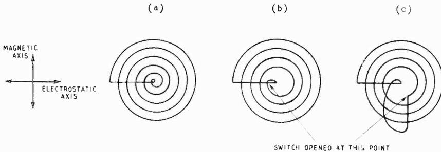
Fig. 2 (left). Forms of trace given by the circuit of Fig. 1: (b) and (c) illustrate the effect of opening the switch at different points of the cycle.
