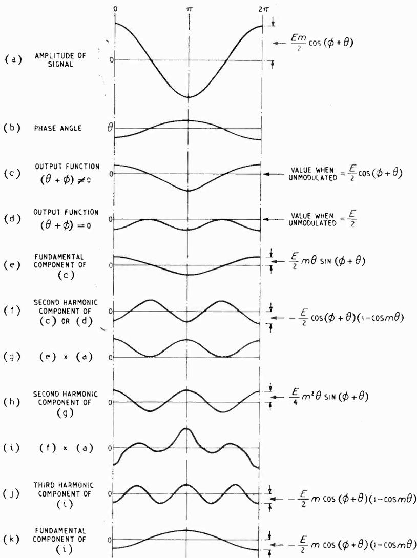
Fig. 2. The analysis of harmonic production is illustrated by this breakdown of the output into its component waves.
