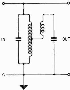
Fig. 2. Tapped-primary circuit.
