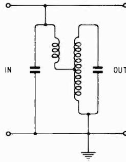
Fig. 3. Tapped-secondary circuit.
