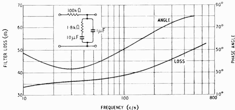
Fig. 8. Calculated performance of RC filter.
