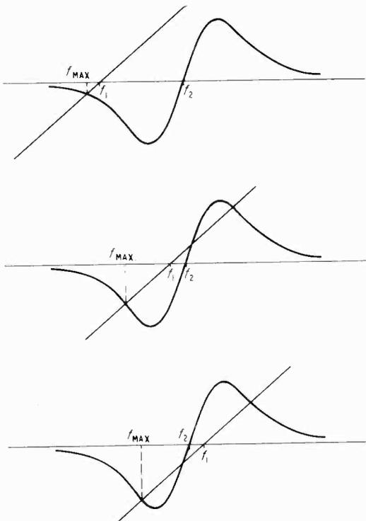
Figs. 10-12. Superimposition of curves of Figs. 6 and 7. Fig. 10 (top) one intersection point only; Fig. 11 (centre)  $f_1$  between  $f_{max}$  and  $f_2$ ; and Fig. 12 (bottom)  $f_1$  on side of  $f_2$  remote from  $f_{max}$ .
