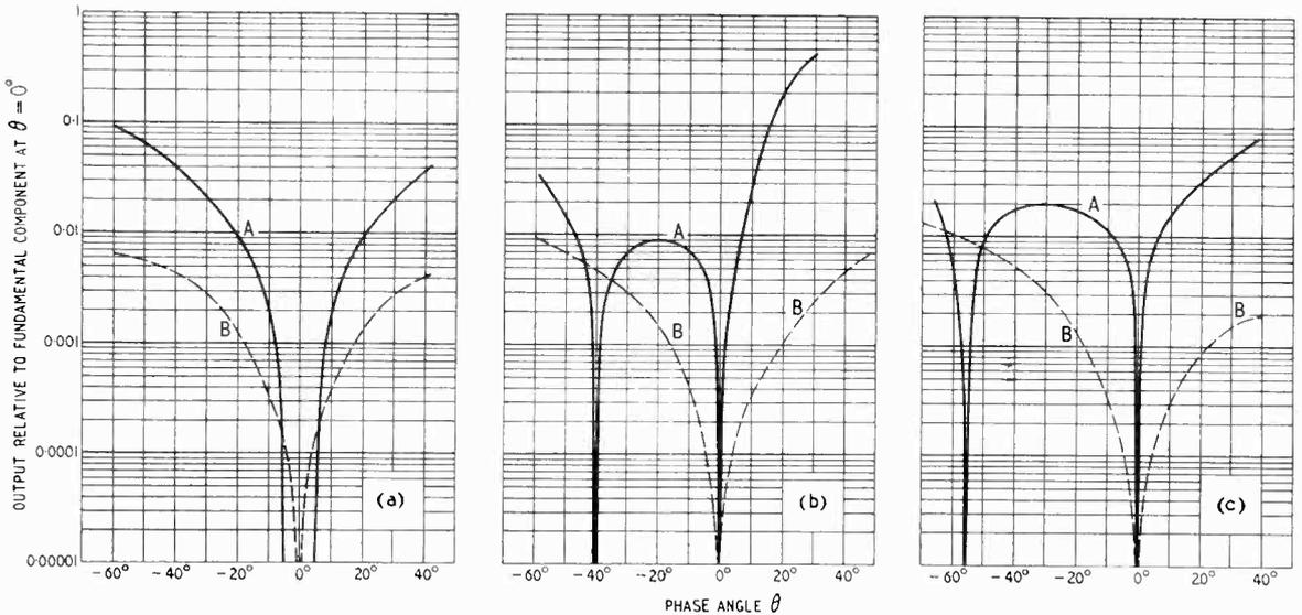
Fig. 4. Output of harmonics of fundamental modulation frequency for  $m = 0.3$ ; (a)  $\phi = 0$ , (b)  $\phi = 20^\circ$  and (c)  $\phi = 30^\circ$ . Curves A and B are for second and third harmonics respectively.
