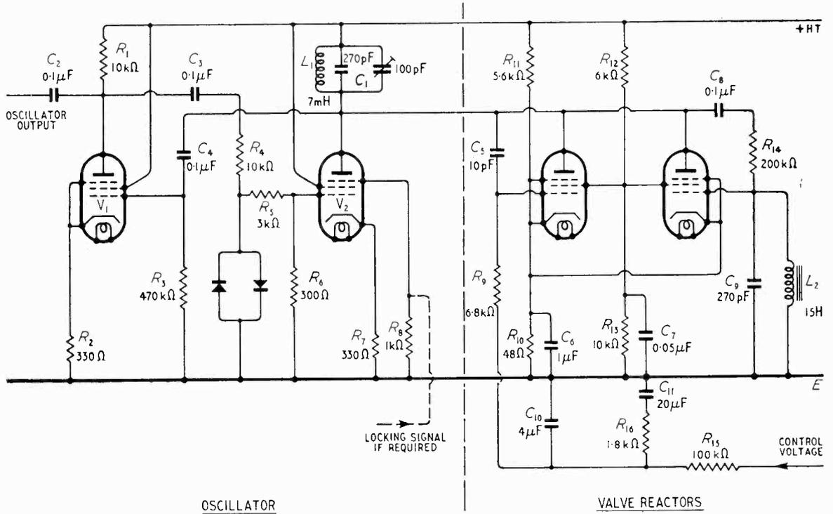
Fig. 7. Oscillator and differential valve reactor circuits. Component values shown are for an operating frequency of 8.4 Kcfs.
