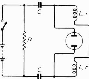
Fig. 1. Basic circuit of spiral time base.
