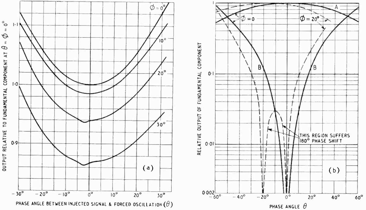
Fig. 3. Fundamental component of modulation frequency ( $m = 0.3$ ); resultant output (a) and components of the output (b). In the latter, curve A shows the main part of the output and curve B the spurious part.
