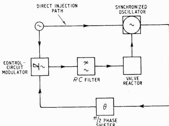
Fig. 6. Phase-control circuit for synchronized oscillator.
