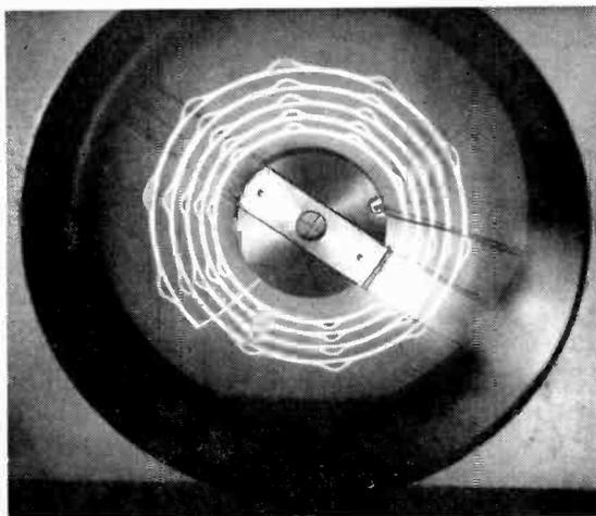
Radial deflection of the trace is obtained by applying the signal to a metal plate fixed to the screen of the c.r. tube.
