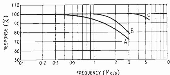
Fig. 17 (above). Frequency response of shunt-regulated amplifier with one stage of inductance compensation. Curve A is the natural response of the Type 2(e) circuit while curve B shows the effect of adding one stage of inductance compensation. The effect of further compensation is shown by curve C.
