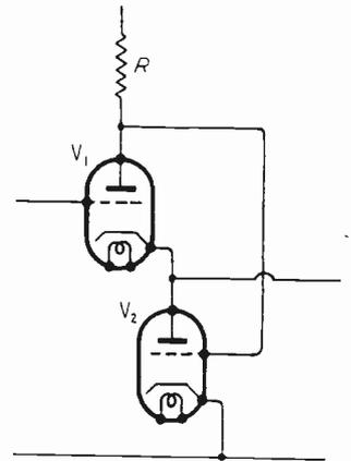
Fig. 6. Shunt-regulated cathode-follower Type 3(e).
