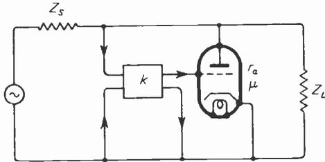
Fig. 2. Circuit of shunt-regulator Type (a).
