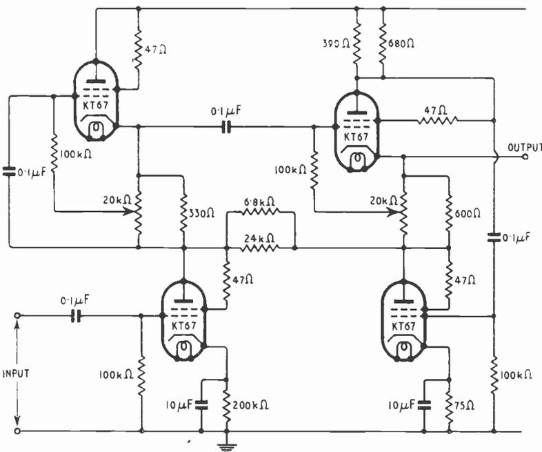
Fig. 15. Experimental shunt-regulated amplifier.
