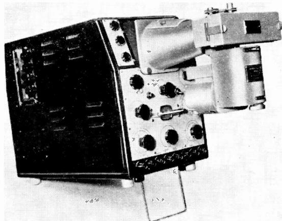
*Cossor 1049 oscilloscope with 1428 camera on 1431 motor drive for camera.*
