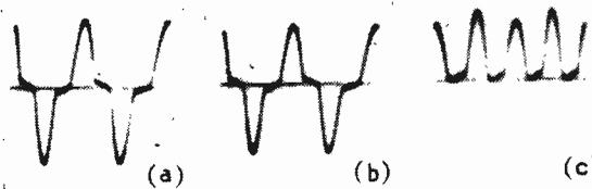
Fig. 4 (above). Oscillograms of currents in a parallel-transductor, Fig. 2 (a).
