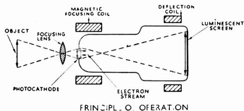
The Image Converters listed below are the first of a comprehensive range at present being developed by Mullard. For full technical information on these tubes, please write to the Communications and Industrial Valve Department.
