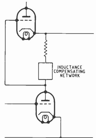
Fig. 16 (above). Method of inductance compensating the feedback resistor.
