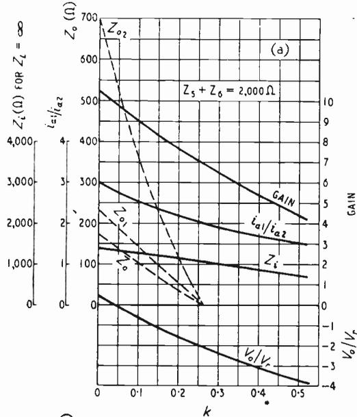
Fig. 10. Characteristics of shunt-regulated amplifier Type 2(e/e);  $\mu = 14$ ,  $r_{a1} = r_{a2} = 600\Omega$ ,  $Z_1 = Z_2 = 100\Omega$ ,  $k = Z_6/(Z_5 + Z_6)$ . The performance for three different values of  $Z_6$  is given in (a), (c) and (d), while (b) gives the multiplying factor for a finite load impedance.
