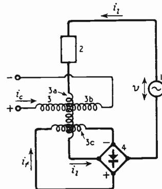
Fig. 1. Principle of a high-gain magnetic amplifier with self-excited transductor. 1. a.c. power supply; 2. load; 3. transductor; (a), load winding; (b), control winding; (c), self-excitation winding; 4. feedback rectifier.
