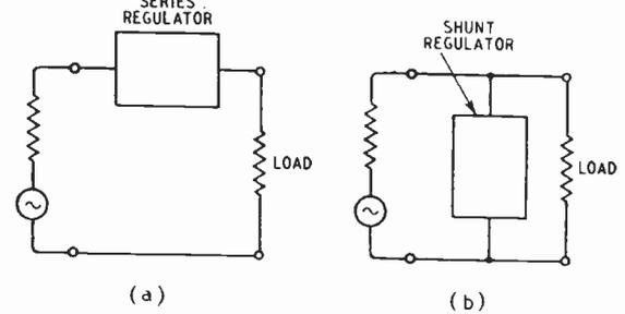
Fig. 1. Basic regulator circuits; series (a) and shunt (b).
