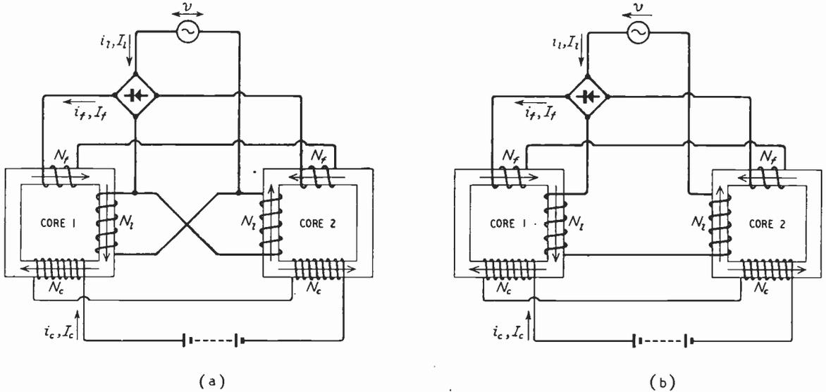
Fig. 2. Transductor arrangement for calculation; (a) parallel-transductor, (b) series-transductor.
