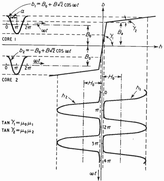
Fig. 3. Magnetic flux densities and magnetizing forces in the transductor cores with a sinusoidal transductor voltage.
