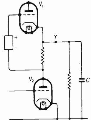
Fig. 5. Shunt-regulated amplifier Type 2(e) with capacitive load circuit.
