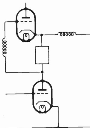
Fig. 18 (right). Further inductance compensation can be applied in the manner shown here.
