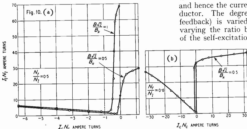
Fig. 10. (a) Large current amplification of a parallel-transducer with  $N_f/N_l = 0.5$ ; (b) small instability loop of a parallel-transducer with  $N_f/N_l = 0.6$ .
