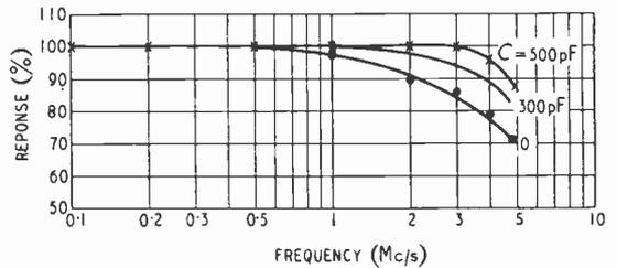
Fig. 14 (right). Effect of load capacitance on the frequency response of the shunt-regulated amplifier of Fig. 15.
