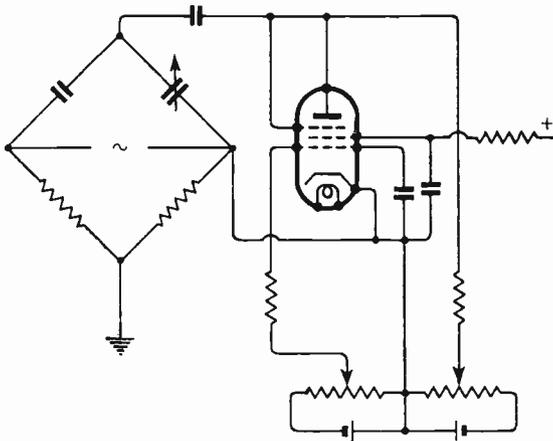
Fig. 10. Method of measuring suppressor-grid to screen-grid capacitance.
