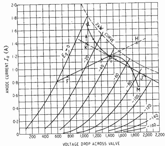
Fig. 8. Characteristics of ACM3 valve with curved load lines due to grid current in the following stage; shunt-regulated cathode-follower Type 3(e).
