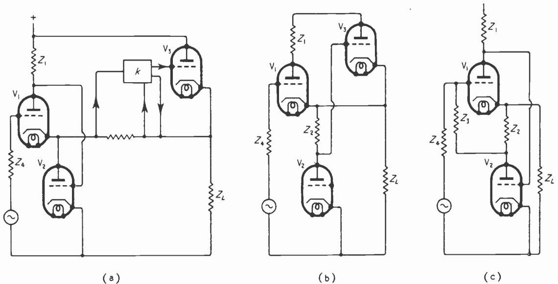
Fig. 12. Derivation of shunt-regulated cathode-follower Type 3(e/e). It comprises a shunt-regulated cathode-follower 3(e) plus a regulator (e) of Table 1. The third valve in (b) can be replaced by a feedback network (c).
