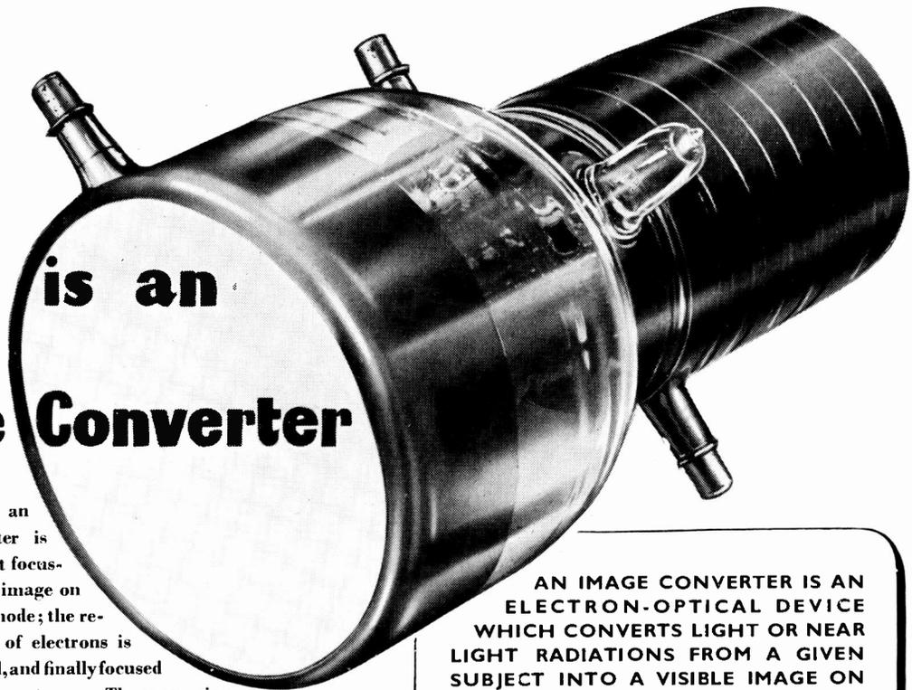
The action of an Image Converter is achieved by first focusing a projected image on to the photocathode; the resultant stream of electrons is then accelerated, and finally focused on to the luminescent screen. The conversion of radiations to electron beams by means of the image converter enables their deflection and modulation by electromagnetic means and thus opens up important new possibilities to designers of electronic equipments. It can, for example, be used for:
