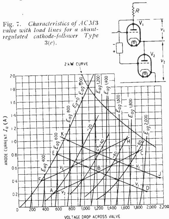
As before, assuming a given instantaneous current flowing through the system with no load connected to the output terminals, and a given h.t. supply voltage, we can derive the grid-cathode excitation of the valve by taking the product of the current and the resistance  $R$ . This settles the voltage drop across the valve  $V_2$  and, therefore, the voltage across the valve  $V_1$ . Current and voltage excursions for the two valves can then be drawn.
