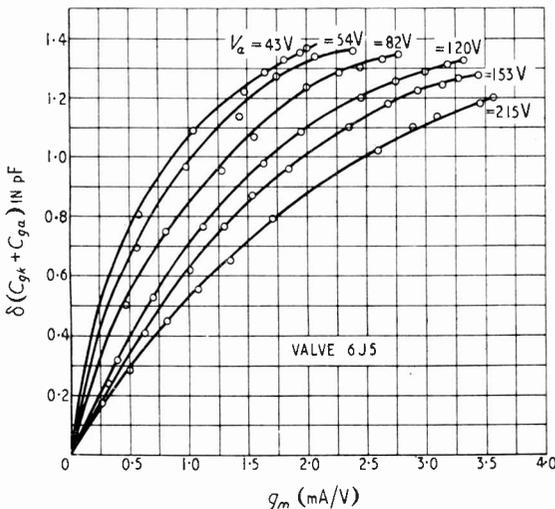
Fig. 3. Variation of capacitance with mutual conductance for a triode.
