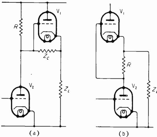
Fig. 3. Circuit of shunt-regulator Type 2(e); general form (a), simplified form for similar valves (b).
