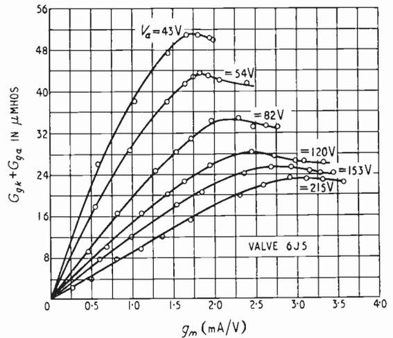
Fig. 4. Variation of conductance with mutual conductance for a triode.
