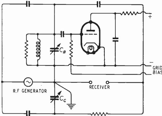
Fig. 2. Twin-T circuit for determining  $\delta(C_{gk} + C_{ga})$  and  $\delta(G_{gk} + G_{ga})$ .
