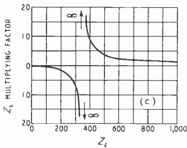
Fig. 13. Characteristics of shunt-regulated cathode-follower Type 3(e);  $\mu = 14$ ,  $r_{a1} = r_{a2} = 6000\Omega$ ,  $Z_1 = Z_2 = 100\Omega$ . The performance with different values of  $Z_4$  is given in (a) and (c) with the input-impedance multiplying factor in (b).
