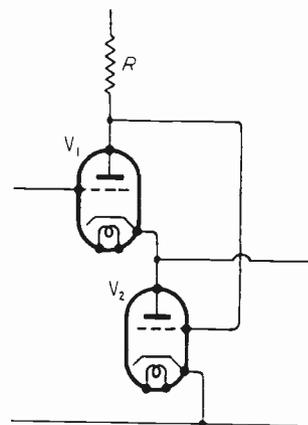
Fig. 6. Shunt-regulated cathode-follower Type 3(e).
