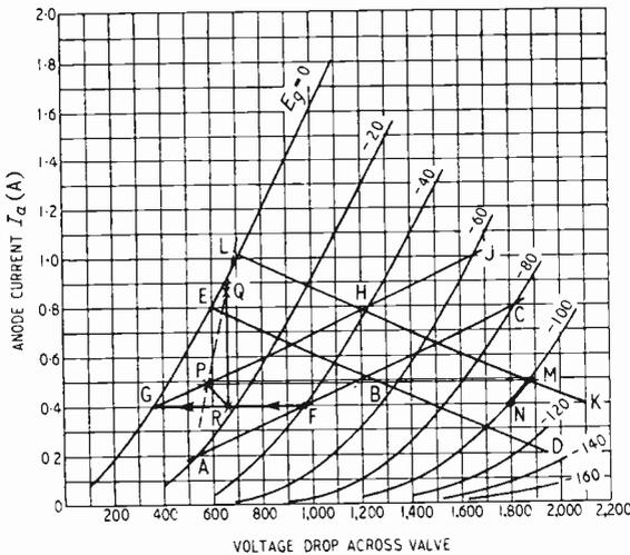
Fig. 4. Characteristics of ACM3 valve with load lines drawn for a shunt-regulated amplifier Type 2(e).
