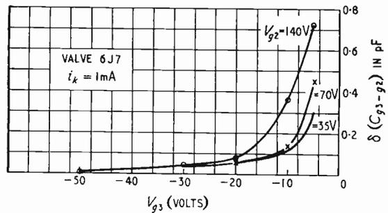
Fig. 11. Variation of suppressor-screen capacitance with suppressor bias.
