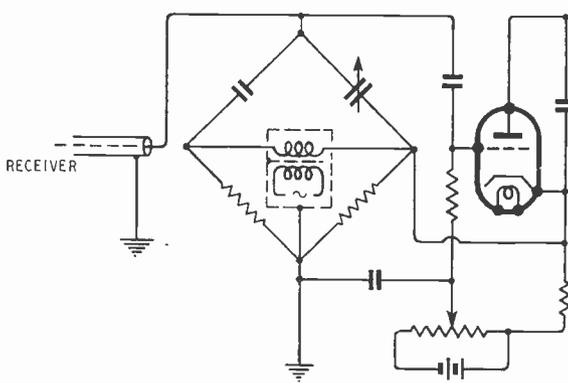
Fig. 1. Method of measuring  $\delta(C_{gk} + C_{ga})$ .
