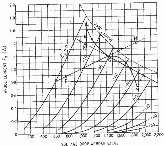
Fig. 8. Characteristics of ACM3 valve with curved load lines due to grid current in the following stage; shunt-regulated cathode-follower Type 3(e).
