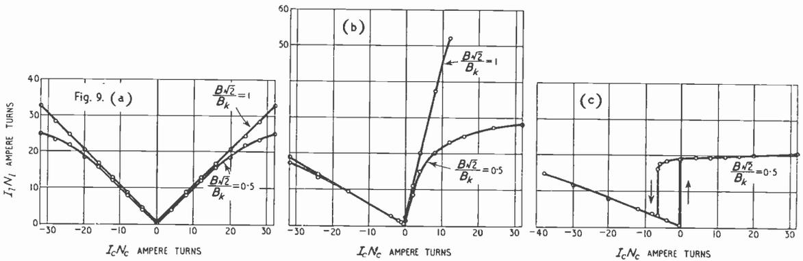
Figs. 6 & 6. Theoretical characteristics of the transducer with  $\mu_1 \rightarrow \infty$  (Fig. 7) and with  $\mu_1/\mu_2 \geq 100$  (Fig. 7); (a) without self-excitation; (b) with low self-excitation (stable region); (c) with high self-excitation (unstable region).
