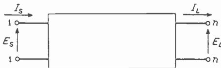
Fig. 1. General representation of four-pole network.
