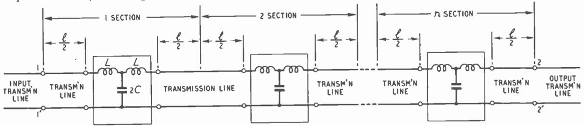
Fig. 8. Example of a  $n$ -sectional periodic structure. (Low-pass filters of Fig. 6 with a length  $l/2$  of a transmission line connected at the input and output of each section.)
