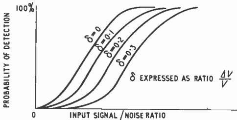
Fig. 2. Probable type of relationship between detection and signal/noise ratio for various values of  $\delta$  (size of j.n.d.) and for fixed values of marking and saturation levels and r.m.s. noise input.
