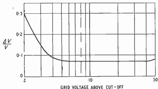
Fig. 1. Typical curve of size of j.n.d. against voltage level for cathode-ray tube.
