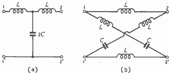
Fig. 6. Example of a T-type low-pass filter (a), and equivalent lattice-type circuit (b).
