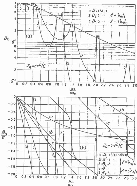
Fig. 10. (a) Magnitudes  $B, B_2, B_3$  and (b) phase values  $\beta/\pi, \beta_2/\pi, \beta_3/\pi$  of the characteristic transmission factors of the periodic structure of Fig. 8 plotted against  $\omega/\omega_0$  for  $\epsilon = 2$  (or  $Z_R = 2\sqrt{L/C}$ ), for  $l = 0$  and  $n = 1$ , for  $l = \lambda_0/4$  and  $n = 1$  and 2, and for  $l = 3\lambda_0/8$  and  $n = 1$  and 3.
