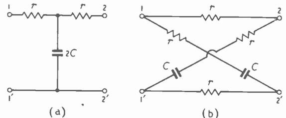
Fig. 11. Example of a symmetrical four-terminal circuit with resistances (a), and its equivalent lattice-type circuit (b).
