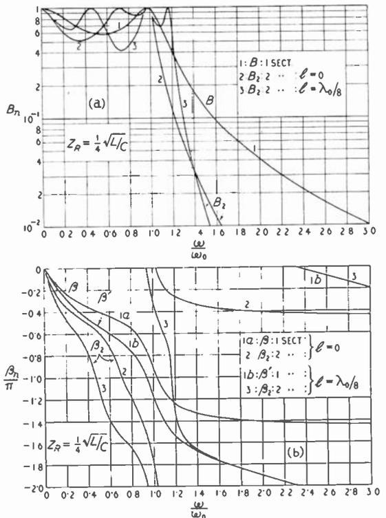
Fig. 9. (a) Magnitudes  $B$ ,  $B_2$  and (b) phase values  $\beta/\pi$ ,  $\beta'/\pi$ ,  $\beta_2/\pi$  of the characteristic transmission factors of the periodic structures of Fig. 8 plotted against  $\omega/\omega_0$  for  $\epsilon = \frac{1}{4}$  (or  $Z_R = \frac{1}{4} \sqrt{L/C}$ ), for  $l = 0$  and  $n = 1$  and 2 and for  $l = \lambda_0/8$  and  $n = 1$  and 2.
