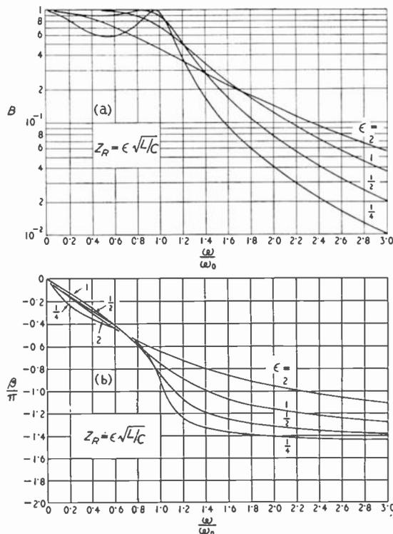
Fig. 7. (a) Magnitudes  $B$ , and (b) phase values  $\beta/\pi$  of the characteristic transmission factors of the low-pass filter of Fig. 6 plotted against  $\omega/\omega_0$  for various values of  $\epsilon$ .
