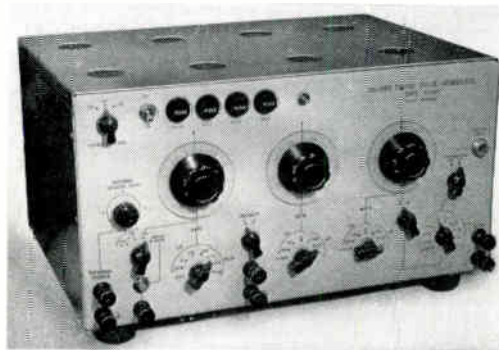
Nagard delayed square-pulse generator, type 5001.
