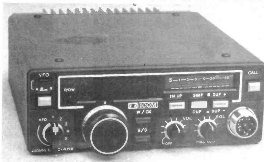
144MHz, with the other response removed by the receive helical filter. Three stages of driver amplification follow, thence to a hybrid PA stage, delivering a stated 25W to the antenna via diode TR switch and low pass filter. While a hybrid stage is convenient for the manufacturers, it may not be such a good idea in the event of it needing replacement.
