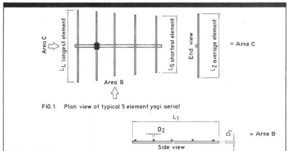
FIG.1. Plan view of typical 5 element yagi aerial
