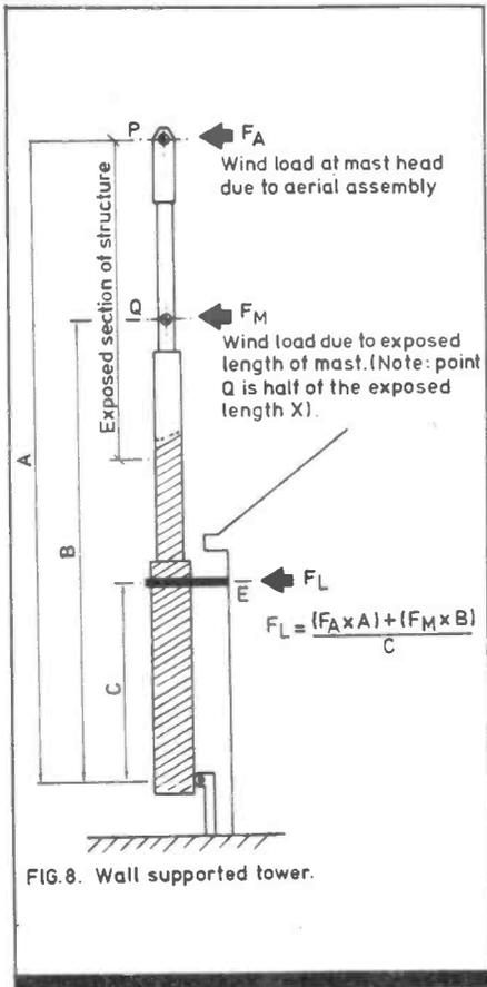
FIG. 8. Wall supported tower.
