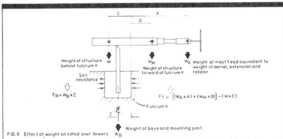
FIG. 9. Effect of weight on tilted over towers
