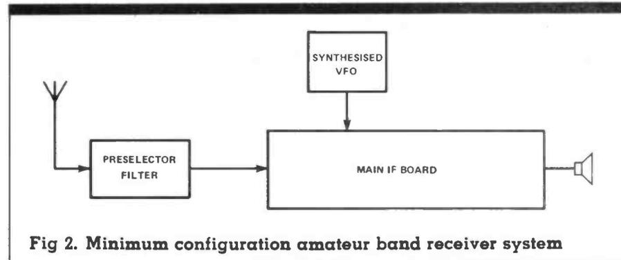
Fig 2. Minimum configuration amateur band receiver system
