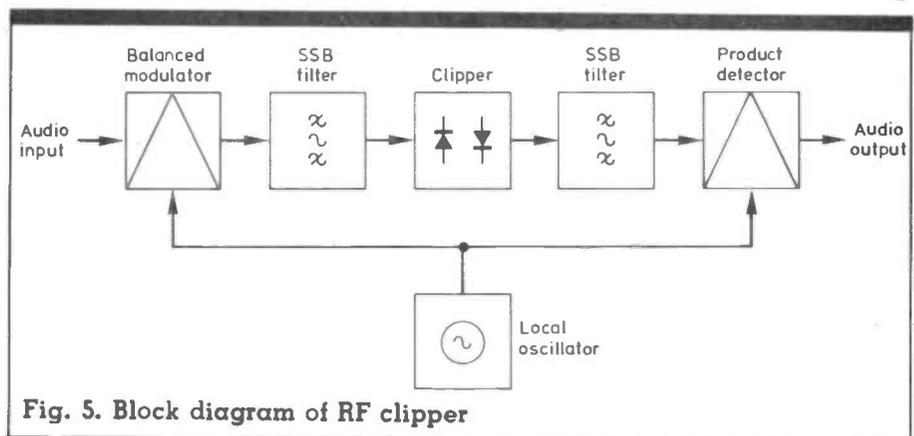
Fig. 5. Block diagram of RF clipper
