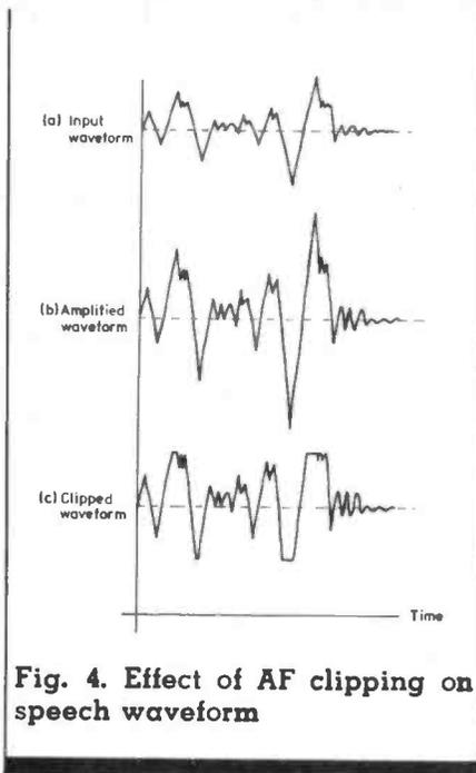
Fig. 4. Effect of AF clipping on speech waveform
