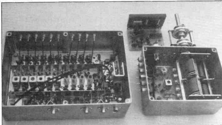
ticlockwise. The reading should start to decrease (showing that the diode is only just conducting). You should set RV3 so that the reading on the probe just limits — at this point the diode is conducting healthily and the output RF voltage will be about 700mV, which is what we want with the frequency display module connected if used.
