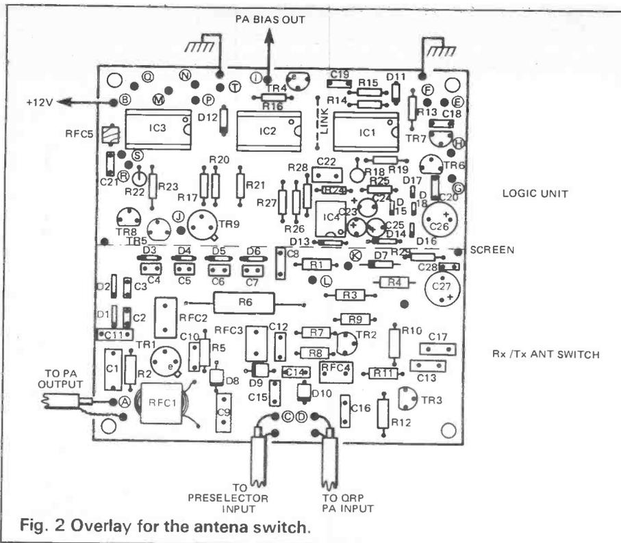
Fig. 2 Overlay for the antenna switch.
