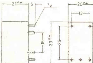
Pre-aligned oscillator block for bias and erase use in cassette and tape decks. High stability push-pull oscillator, with shielded case.
