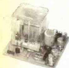
Very substantial 20A relay driven by the multifarious HA12002 amplifier monitor IC. Protects against overload, temperature offset etc.
