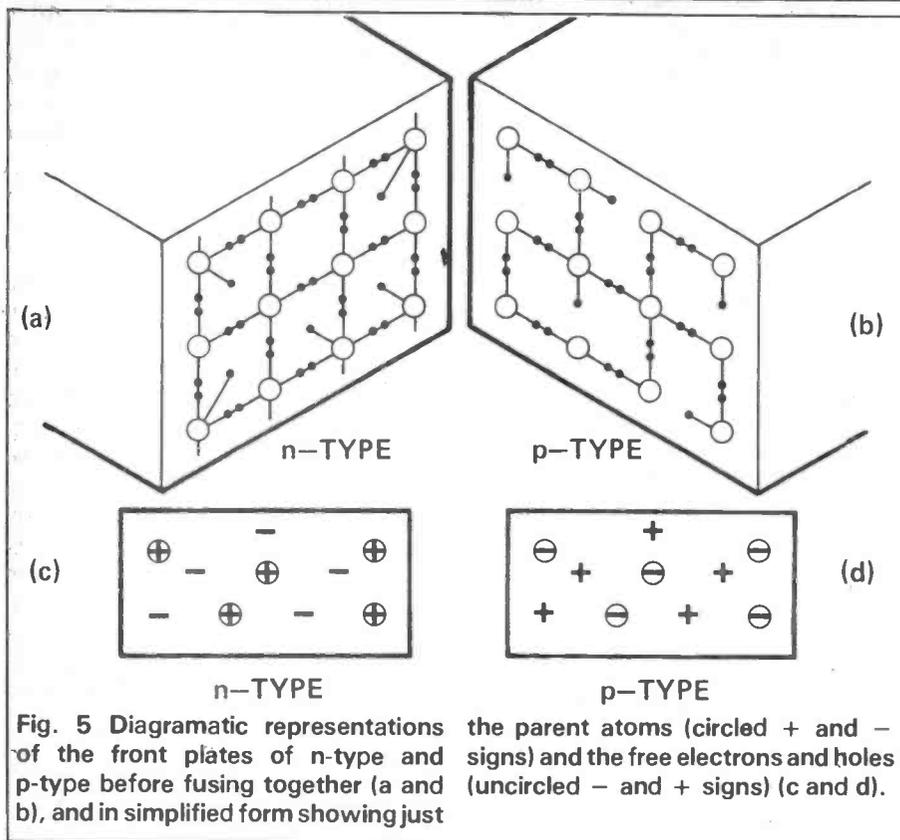
Fig. 5 Diagrammatic representations of the front plates of n-type and p-type before fusing together (a and b), and in simplified form showing just the parent atoms (circled + and - signs) and the free electrons and holes (uncircled - and + signs) (c and d).
