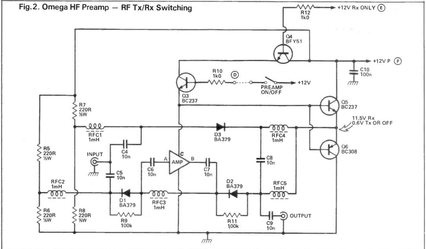
inhibit parasitics associated with the transformer leakage inductances. The amplifier provides a flat gain of 15dB across the HF spectrum when correctly terminated on both input and output into 50 ohms. It has an output capability of +15dBm (about 30mW).
