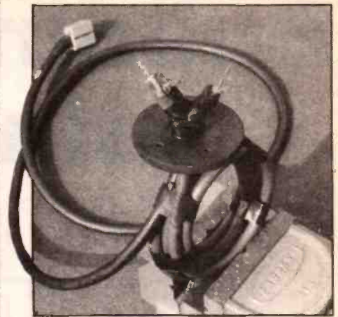
The phasing sections of the 10m crossed dipole should be coiled up and fixed with tape.
