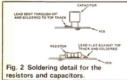
Fig. 2 Soldering detail for the resistors and capacitors.
