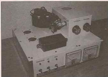
50MHz legal limit amplifier, including power supply and 500WV low pass filter, there's a full construction article on the way this winter for Ham Radio Today!
