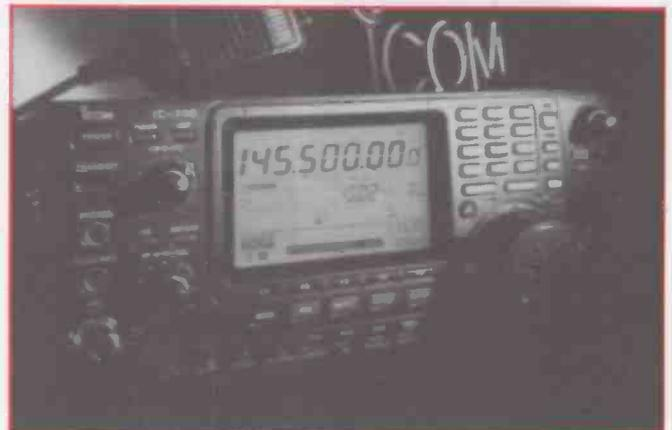
to-read function display, the IC-746 indicates standard details like operating frequency and memory channel number, as well as function settings and digital meter indications. However, in order to provide all essential information at a glance, the display also features a multi-function dot matrix screen which registers the 'bandscope' settings, twin PBT settings, split frequency operation modes and the contents of the memory keyer.
