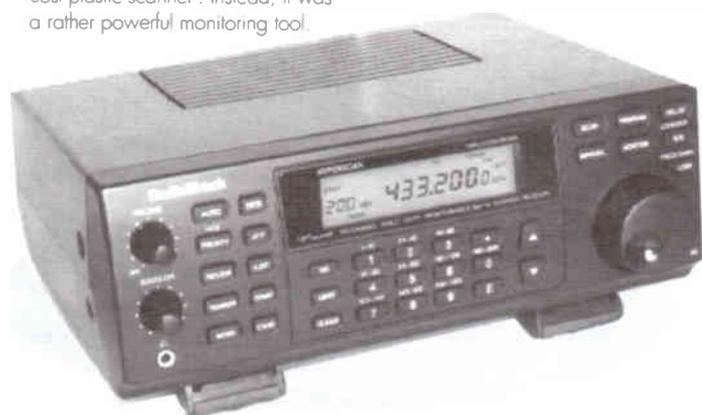
The PRO-2045 measures 57mm x 235mm x 205mm and weighs 960g. A pair of hinged plastic feet at the front of the case lets you tilt up the front of the set for table-top use.
