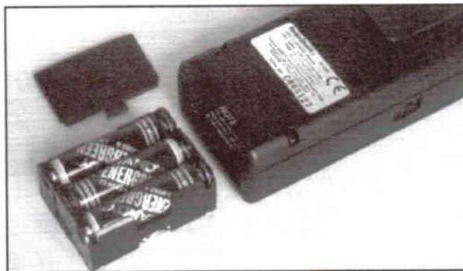
**Six AA batteries are used for power, these fit into a battery pack which slides into the case**
