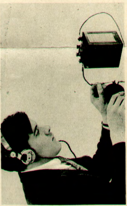
Fig. 7. Continuity of winding in a high-frequency plug-in transformer is tested by making connexions to opposite legs. A click will be heard if the windings are sound
