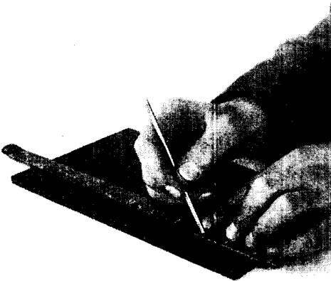
Fig. 3. Draw a line accurately at right angles to the first two. It is important that the panel be first marked out, or the work may be spoiled
