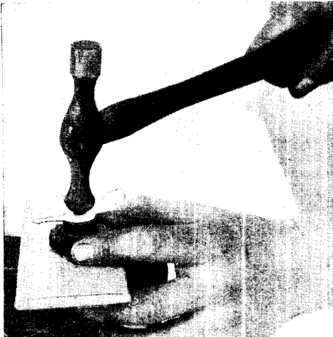
Fig. 3. Riveting is sometimes adopted as the method of attaching a pointer to a knob. A tubular projection is added to the knob
