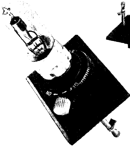
Fig. 15. The Holderstat is fitted with a valve. This panel combines the functions of a filament resistance and a valve holder in one
