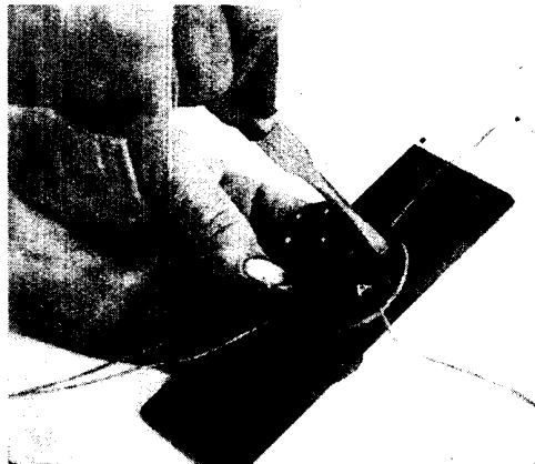
Fig. 4. Under a valve holder rubber packing is placed as a means of reducing vibration and the microphonic noises which often result
