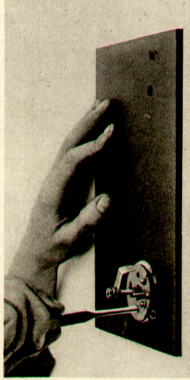
Fig. 5.—Holes are drilled in the panel for fitting the filament resistances. One is shown in position
