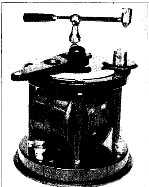
Fig. 1. The McMichael crystal set provides efficient reception inside a radius of 10 to 15 miles from a broadcasting station
