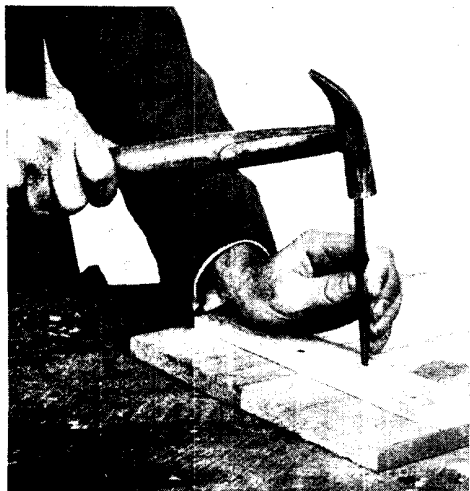
Fig. 4. Nails are being driven below the surface of the woodwork by using a nail-set punch
