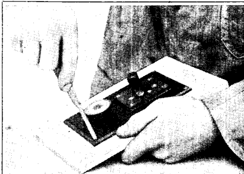
Fig. 13. When the stud switch and filament resistance have been mounted the panel is secured to the wood front
