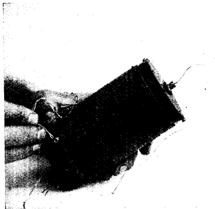
Fig. 14. Winding is completed by taking the wire through the former after the last turn
