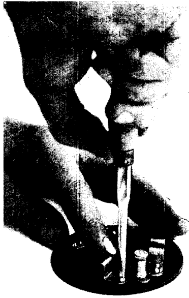
Fig. 1. In the complete swivel switch a ball and socket joint gives quickly any of three desired contacts
