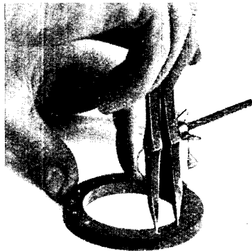
Fig. 9. Marking the ring for positions of the contact studs leading to tappings
