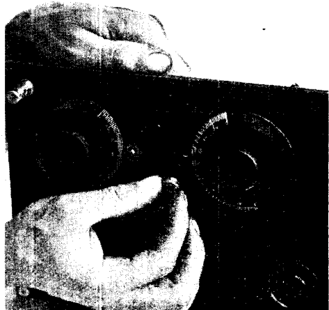
Fig. 5. Here the panel holes are drilled and counterbored to receive the vernier control shown in Fig. 4
