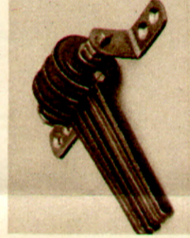
Fig. 11. Here are shown the two basket coils, forming the aerial coil and reaction coil, and the spade-tuning plate used in the receiver
