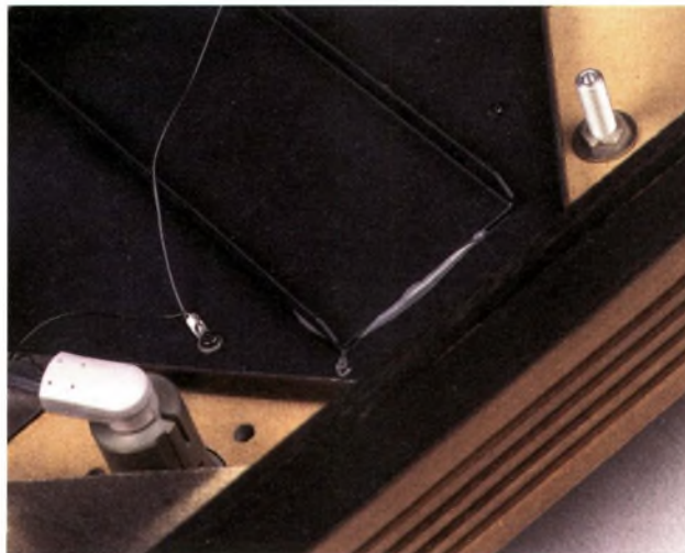
Underside of sub-chassis showing later glued construction.
