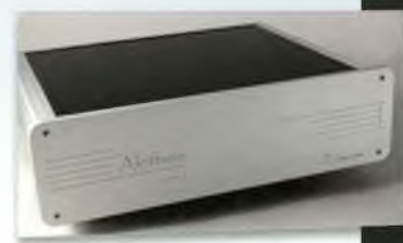
Aletheia PSU2 power supply has Vertex energy control and RFI/EMI shielding applied right down to individual circuit components.
