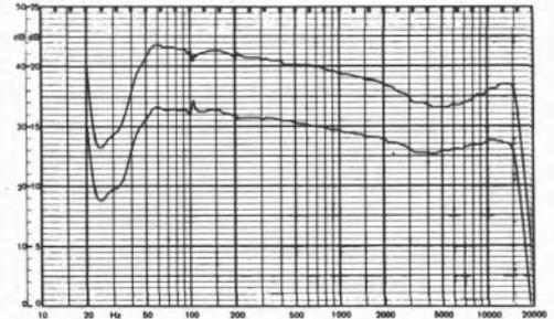
This deck does not include a Dolby noise reduction system, but has instead Philips DNL for replay only, which frankly serves purely as a hiss remover whilst unfortunately removing much of the sheen of quiet music as well. The overall noise performance was extremely good and indeed marginally superior to almost all machines incorporating Dolby but with the Dolby circuit not operating.
