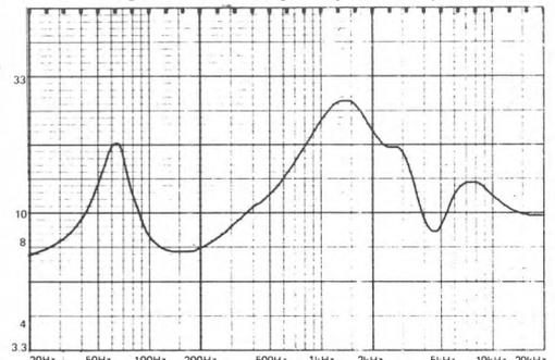
below: averaged frequency response at 2m (solid curve on axis, dotted curve  $10^0$  vertical, dashed curve  $30^0$  horizontal) vertical scale 1dB/div.
