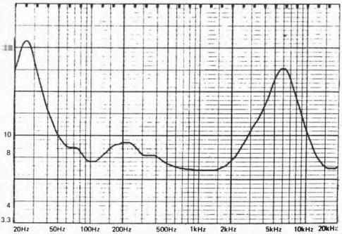
below: averaged frequency response at 2m (solid curve on axis, dotted curve  $10^0$  vertical dashed curves  $30^0$  horizontal, curve marked + represents second sample).
