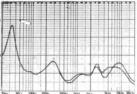
below: averaged frequency response at 2m (solid curve on axis, dotted curve 10° vertical dashed curves 30° horizontal L&R) vertical scale 1dB/div.
