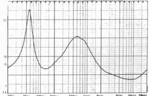
below: averaged frequency response at 2m (solid curve on axis, dotted curve  $10^\circ$  vertical dashed curves  $30^\circ$  horizontal L&R) vertical scale 1dB/div.
