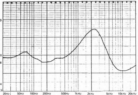
below: averaged frequency response at 2m (solid curve on axis, dotted curve  $10^\circ$  vertical, dashed curve  $30^\circ$  horizontal) vertical scale 1dB/div.
