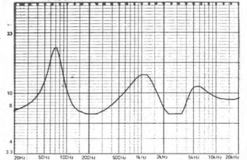
below: averaged frequency response at 2m (solid curve on axis, dotted curve  $10^\circ$  vertical, dashed curve  $30^\circ$  horizontal) vertical scale 1dB/div.
