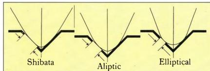
It is basically elliptical (.0003" x .0007"), but its bottom radius has been modified to extend the vertical bearing surface on the groove wall by 100%.
