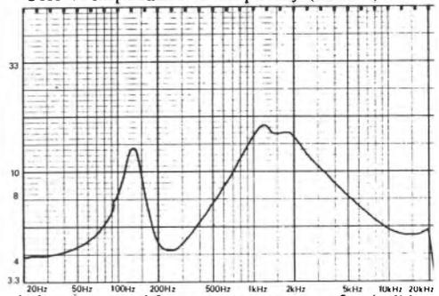
below: averaged frequency response at 2m (solid curve on axis, dotted curve  $10^\circ$  vertical dashed curves  $30^\circ$  horizontal L&R) vertical scale 1dB/div.
