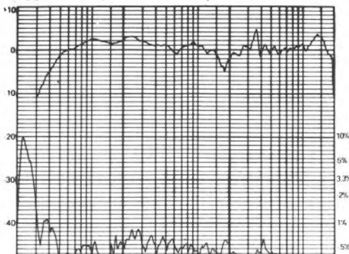
below: averaged frequency response at 2m (solid curve on axis, dotted curve  $10^0$  vertical, dashed curve  $30^0$  horizontal) vertical scale 1dB/div.
