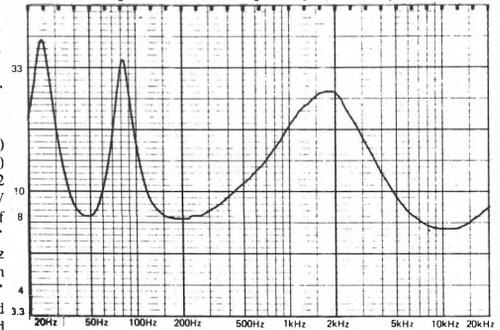
below: averaged frequency response at 2m (solid curve on axis, dotted curve 10<sup>0</sup> vertical, dashed curve 300 horizontal) vertical scale 1dB/div.
