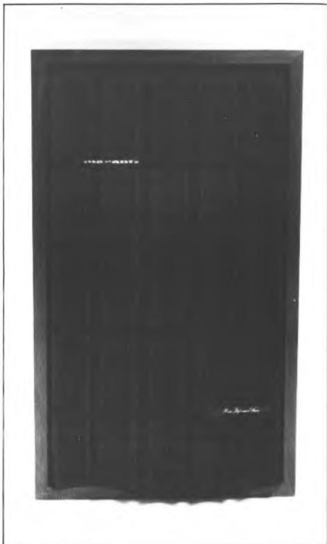
This Marantz loudspeaker is built in Belgium, and in addition to its unusual sculpted foam front, it offers further interesting features. Three response controls are provided for treble, mid and bass registers. The latter consists of a thick foam plug with an attached handle, that can be used to block the large ducted reflex port and thus convert the speaker into a sealed-box enclosure, with more extended bass at a reduced level.
