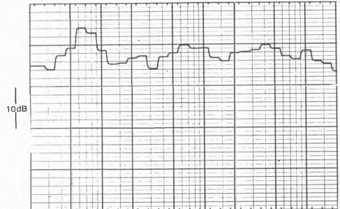
Averaged forward characteristic response in room at listening position.
