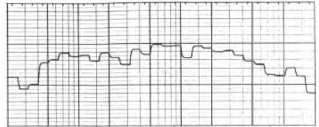
Averaged forward characteristic response in room at listening position.
