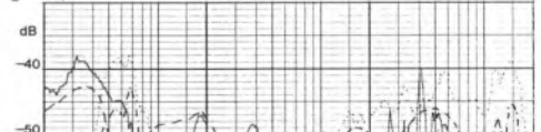
Harmonic distortions: solid 3rd 96dB, dotted 2nd 96dB, dashed 3rd 90dB, chain-dashed 2nd 90dB, ○ shows stop point at 96dB).
