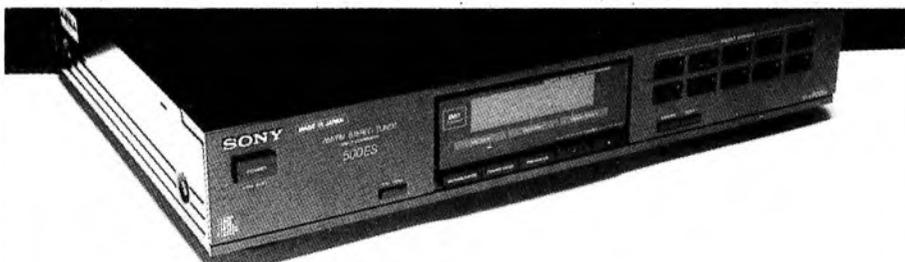
In our last tuner tests, the 500ES' more expensive 700 stablemate was very well liked. The 500 is also a digital synthesiser design, has very similar styling and equally good finish and substantial build, but lacks some of the 700's facilities.
