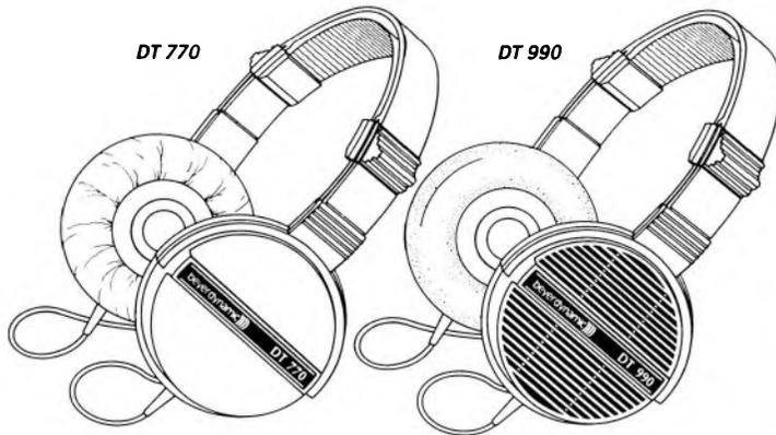
The DT 770 closed headphone combines the latest transducer technology with a unique bass reflex system. This achieves a superb bass response with well defined sound image, plus excellent pulse characteristics.
