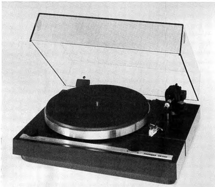
The TD320 is the top model in Thorens' new series, and is also available without arm (321). Following in the footsteps of B&O and Philips, Thorens have chosen to replace their usual coil spring suspension with one using flat leaf springs, these hung or cantilevered from the chassis allowing free movement. Centration and consistency are thus improved and the springs are easy to adjust from above.
