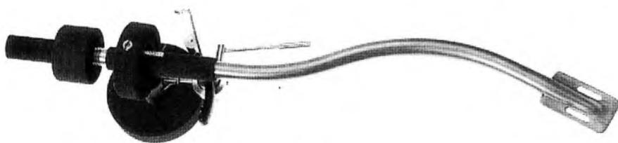
Apart from the black finish used on all parts aft of the armtube, it's hard at first to distinguish the *Xenon* from its more expensive *HR-100S* stablemate. The *Xenon* armtube and headshell is the same one-piece fabricated titanium component, damped internally and without any structural break until quite close to the bearings.
