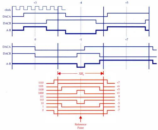
Figs 4a (top) and 4b: JVC's PEM D-to-A converter.
