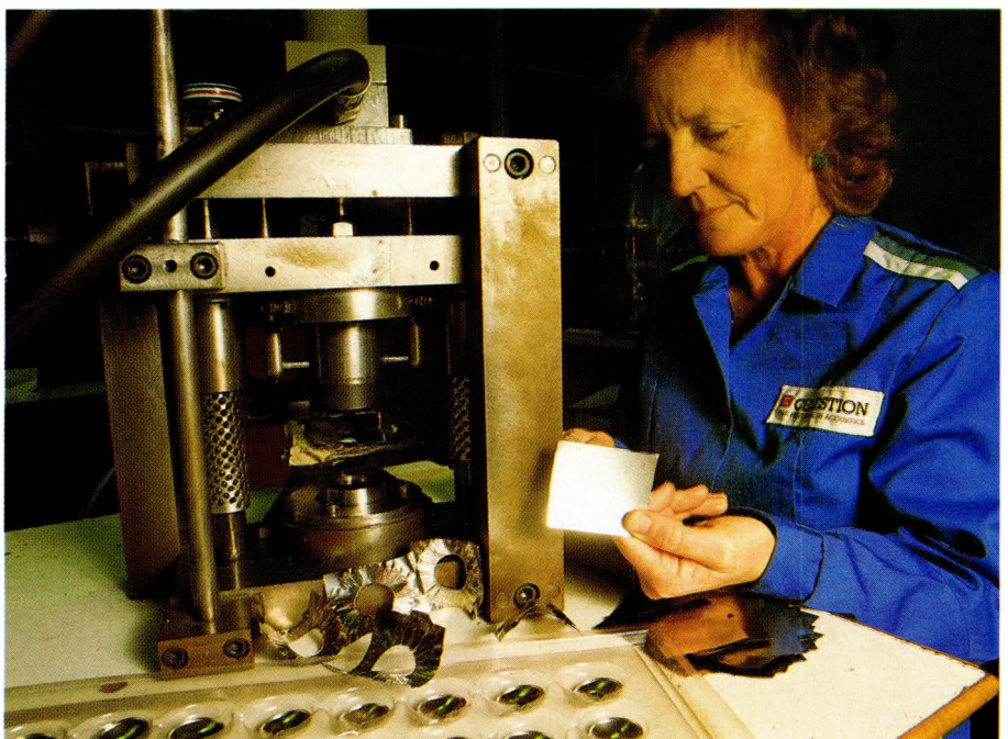
Half a metre of 11mm wide wafer thin aluminium ribbon is handcrafted onto its jig.
