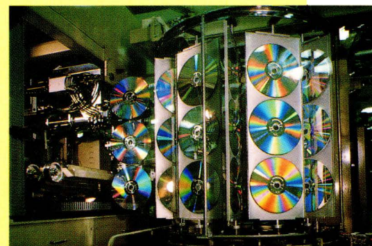
Completed discs leave the metallising chamber complete with their reflective surface.
