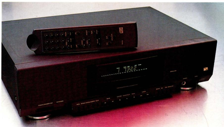
After months of expectation Philips' has gotten around to utilising its own two-chip Bit Stream DAC — the fabled DAC7. Not that the sober exterior of the CD950 gives any hint to the treasure lying within. In terms of styling the CD950 is hot from the 900 Series mould, it even has the same display and CDM9 transport mechanism as the budget CD930. To be perfectly fair, however, Philips has tarted-up its CD drawer with a soft covering of felt.
