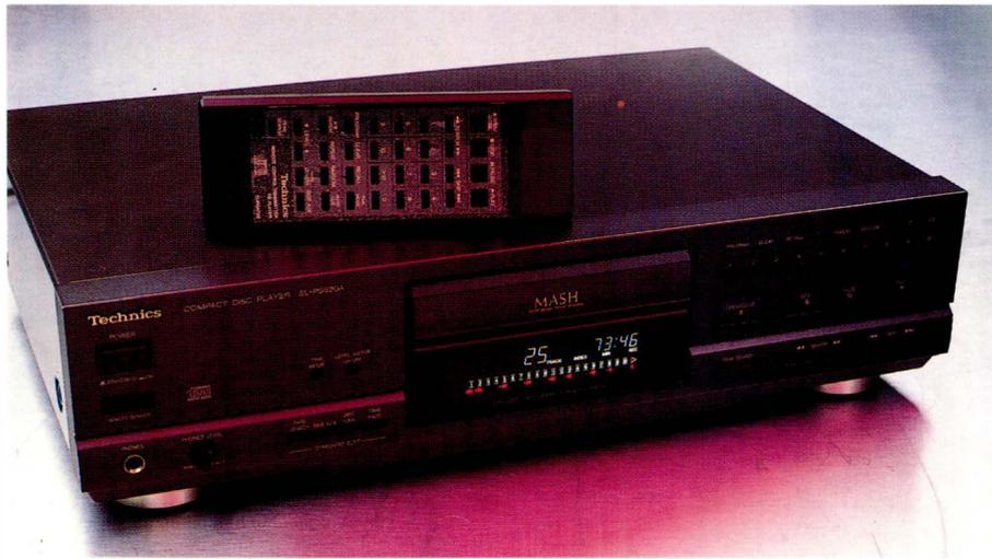
**T**echnics has made a valiant attempt to disguise the origins of its SL-PS620A. But just as the SL-PG320A is inextricably linked to the SL-PG420A, so too is the SL-PS620A bound to its cheaper sibling, the SL-PG520A. Basically, the 520's digital gubbins have up and moved house into a fresh new case, complete with an anti-resonant base and very swish matt-bronze fascia.
