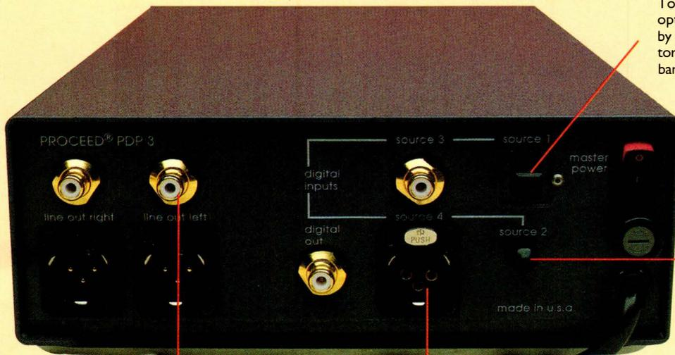
Toslink: the de-facto optical standard, limited by its snap-fit connectors and restricted bandwidth (speed).
