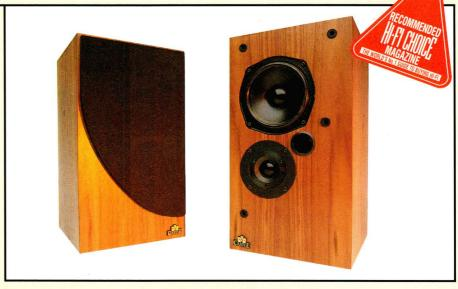
high class finish and flush mounted drivers. The box itself feels reassuringly solid. It's built up from 16mm MDF wrap plus a 19mm baffle, and the panels are damped/mass-loaded by bituminous pads, further lined in absorbent foam and with a final additional box-volume fill.
