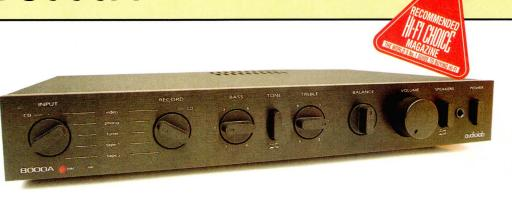
In truth the basic topology of the *8000A* is now ten years old but significant changes to the board layout, earthing, power supply and choice of components keeps the *8000A* sounding fresh. Elna Duorex signal-coupling capacitors were changed for Starget electrolytics for issue 129 while, one year on, a new mains transformer, ground reference and a two (rather than three) wire mains connection has brought the *8000A* into line with new European safety standards (including EN60065 and IEC65).
