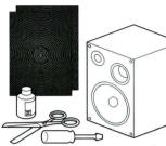
Once you have gained access to the inside of the cabinet, remove foam and/or wool damping from the inside of the speaker (if fitted)
