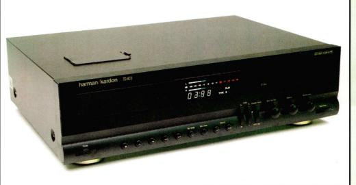
The *TD420* is a horizontal drawer-loading design, and has a very clean facia with a bare minimum of controls and a large, clear but simple display panel.
