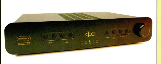
there's even a switched headphone socket mounted on the rear panel — alternatively this can serve as a preamp output to drive DPA's matching *Renaissance* power amps.
