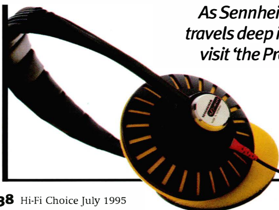
The HD424, one of Sennheiser's earliest models, was based on the 'open air headphone' principle.
