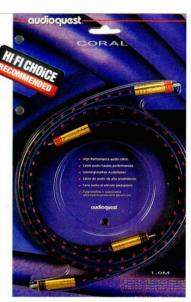
This classic solid-core cable has been in production longer than most, and what you see is what you get: two thin solid copper conductors, identical but for the colour of their insulation, spaced apart by a 'web' of polythene, with no screening, for £40/m-pair. The phono plugs were chosen because they have less metal in them than most other types.
