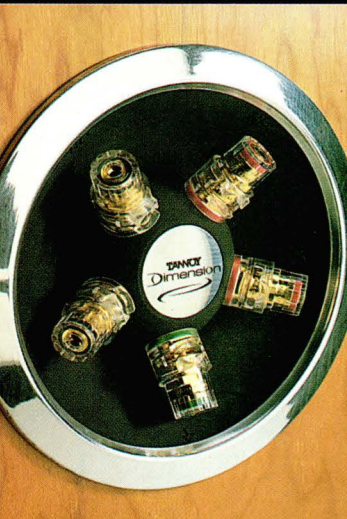
Above: the black area is actually velvet for minimal cabinet reflection of the super-tweeter's output. Right: the device itself sits in a solid aluminium billet that is earthed to the fifth terminal (below) in order to reduce the effects of RF interference on voice coils.
