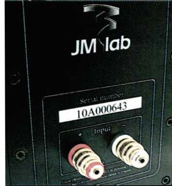
Above: Bi-wiring and bi-amping are eschewed in favour of a single set of high-grade terminals and a state-of-the-art crossover.
