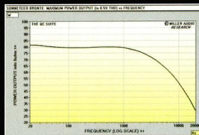
The amplifier will deliver 2x80W/8ohm and a full 2x125W/4ohm at 1kHz at less than 0.5% distortion. Nevertheless, because distortion increases quite markedly with frequency, there's progressively less 'clean' power available through the upper midrange and treble. At 20kHz, and the same 0.5% limit, power output is down to just 30W/8ohm.
