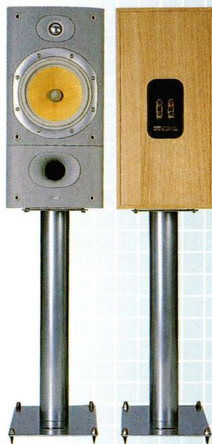
New light grey mouldings ginger up this timeless design. A metal dome tweeter features Nautilus-style tube loading, while a relatively large bass/mid driver has a shiny cast frame, Kevlar cone and grey rubber surround. The front-mounted port is gas-flowed and stippled to avoid turbulence.
