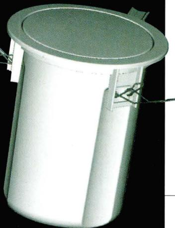
**KEF** has a new custom installation loudspeaker, the Ci100QR. Built for flush mounting into walls and ceilings, the speaker uses a Uni-Q drive unit comprising 100mm polypropylene bass driver and a 19mm tweeter. Its 0.7 litre enclosure is said to offer optimum low frequency reproduction and the unit can be fitted to walls varying in thickness from 6mm to 30mm. Expect to pay £100.
