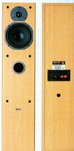
A simple two-way with a modest size bass/mid driver, this very compact floorstander is really more like a standmount with its own integral stand, since only the top half of the enclosure is acoustically active. Mass loading may be added to the base for improved stability.
