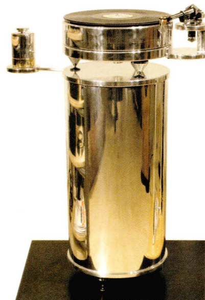
Small Royal, 60cm aluminium platter, topped with a 6mm acrylic platter and leather mat. Nylon thread belt - weight 25kg, rrp £1280 without tone-arm. (TT shown with Type Two Stand)
