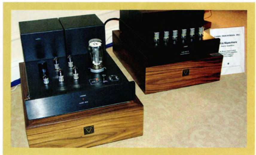
Right: 32 single-ended watts are all you get from this, just one channel of the Lamm ML3 signature and its huge outboard power supply
