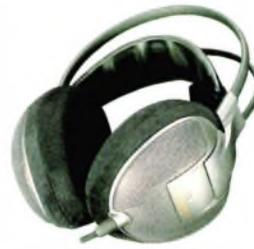
Headphones come in several varieties and some are designed for particular usage. The majority of 'cans' use dynamic cone and coil-type drive units and can be used with anything from a personal stereo to a dedicated amplifier. Other types also exist, most significantly electrostatics that use a charged panel membrane to produce a distinctly refined sound. These are supplied with their own dedicated amplifiers, which tends to increase the price.
