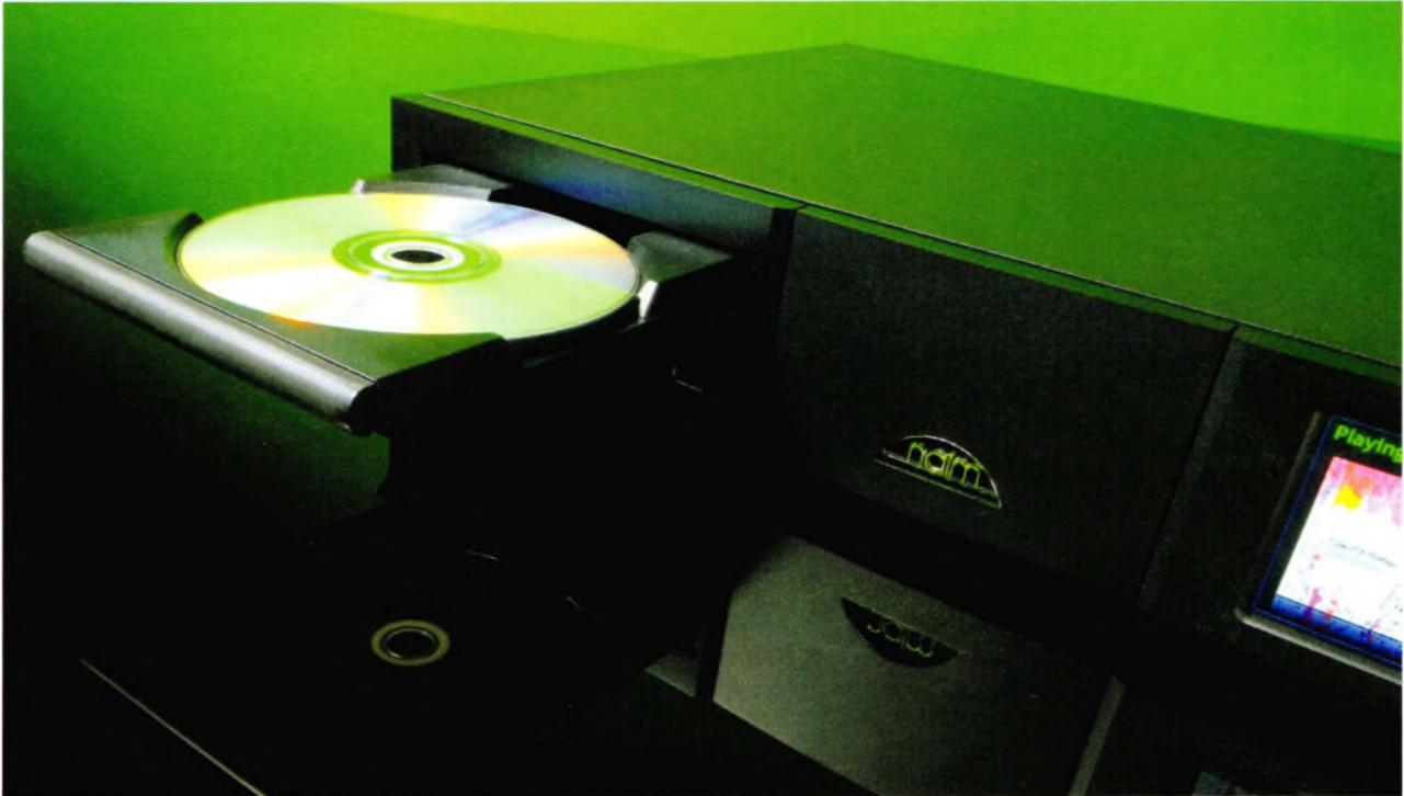
used to create bit-perfect copies of the CDs fed into the front-panel drawer. Rather than rely on the widespread 'burst mode' ripping technology, which is prone to introducing and perpetuating errors, the Naim ripper works more methodically, reads discs multiple times and uses no caching to ensure you get replay that's free from inaccuracies or time offsets.
