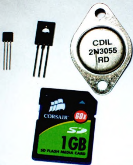
Above: The many faces of the transistor. Top: (left to right), single transistors for small-signal, medium-power and high-power use. Bottom: several billion transistors in an SD memory card.'
