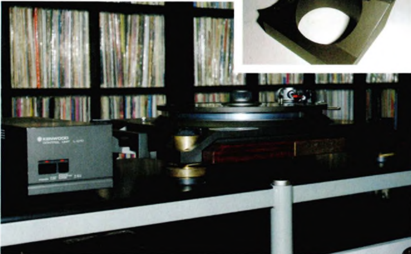
(Above) Richard Kunz's deck with Kenwood centre weight, periphery clamp and unpainted feet
