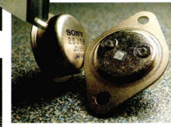
(Right) Inside a 2SJ18 V-FET from the TA-N7B linear amp
